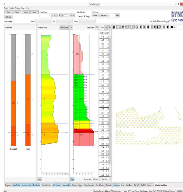
The system can load up to four distinct segments in each blasthole in a single pass. Measurement While Drilling (MWD) data is captured and set to a specific energy requirement using ΔE<sup>2</sup> software, to optimise design with the required energy placement in each blasthole. The aim is ultimately to improve the overall blasting outcomes.
